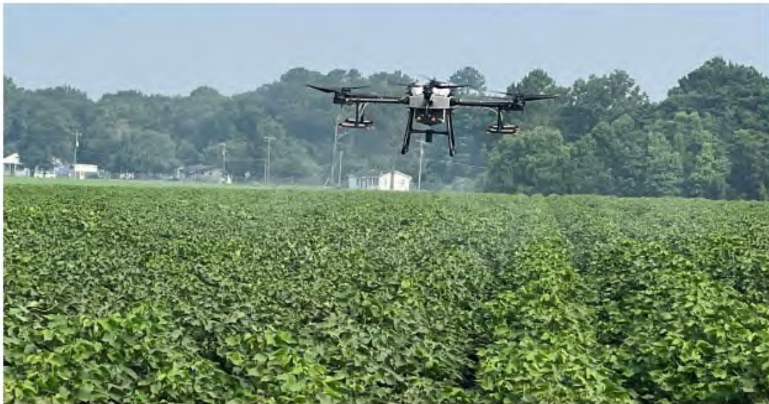
Fungicide application with DJI AGRAS T30 spray drone in cotton
